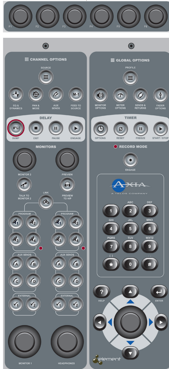
Figure 4-4: Master Module + SoftKnobs
