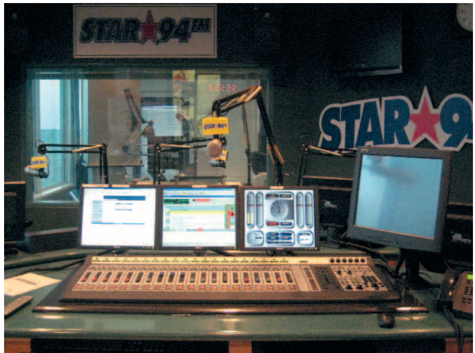
The Axia control surface at WSTR with controlling software visible on screen.
